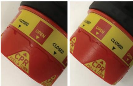
has been released, remove patient from mattress, turn the cap in either direction by one notch to the 'CLOSED' position. Ensure control unit is switched on, press MAX INFLATE and wait for the system to regain pressure.
